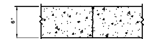
6 TYPE 'H' CONSTRUCTION JOINT DETAIL C5.0 NOT-TO-SCALE
